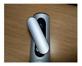
The device may power on when you connect the USB. If it does not, press and hold the button on the top center of the device.
