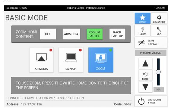
2. To enter into the ZOOM interface on the touch panel, press the Home Icon located at the top right of the touch panel.
