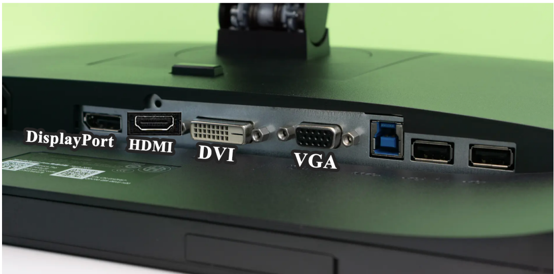
This monitor has from left to right: DisplayPort, HDMI, DVI and VGA ports.
