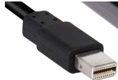
Dell DisplayPort (DP): Note it is asymmetric
